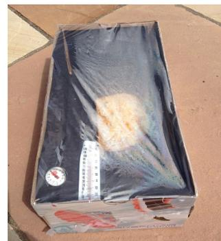
Set up the controls as well. Set up thermometers in each one, and one thermometer in a sunny location outside the oven (regular thermometers are fine for the controls, since these won't get very hot).
