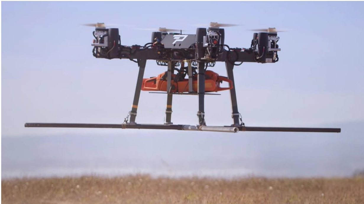
Prototype Parallel Hybrid Multirotor in flight with 18kg (40lbs) of payload.
