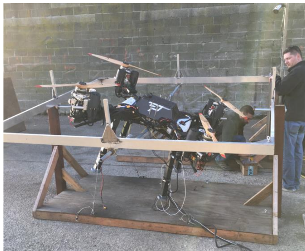
Prototype aircraft on a test stand used to demonstrate fault tolerance using a novel clutch mechanism.
